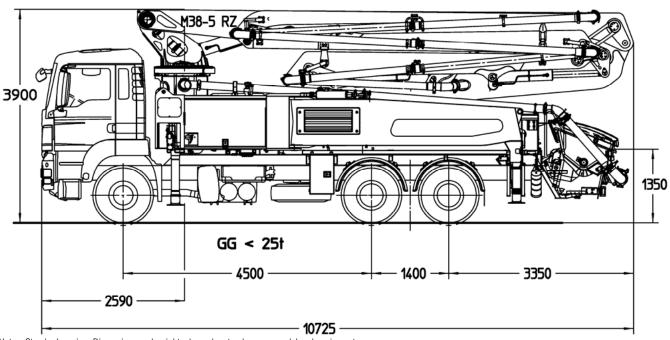
Note: Standard version. Dimensions and weights depend on truck, pump model and equipment. Dimensions in mm, MAN TGS 26.400.
